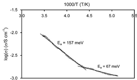
**Fig. 5** Conductivity as a function of reciprocal temperature for electrodeposited  $[(n\text{-C}_4\text{H}_9)_4\text{N}]_2[\text{Ni}(\text{dcbdt})_2]$ .
