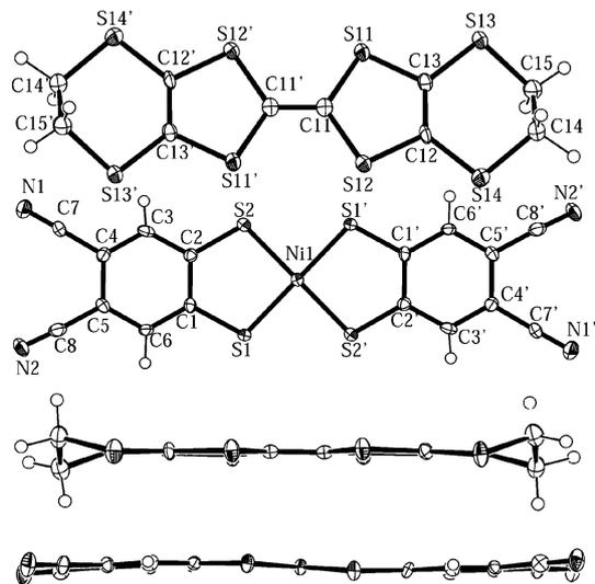
**Fig. 7** Molecular structure of BEDT-TTF and Ni(dcbdt)<sub>2</sub> in (BEDT-TTF)[Ni(dcbdt)<sub>2</sub>] (top: onto the plane of the molecules; bottom: side view of the molecules).
