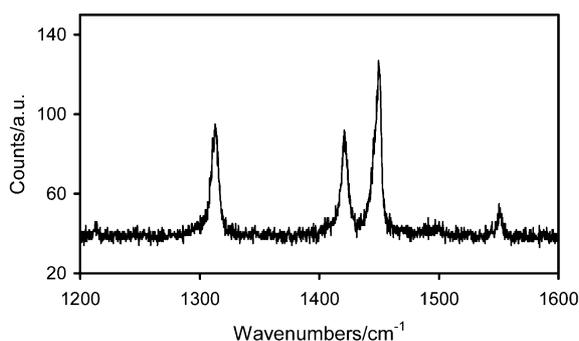
**Fig. 8** Raman spectrum of electrodeposited thin films of (BEDT-TTF)[Ni(dcbdt)<sub>2</sub>] ( $\nu_{CC}$  region).
