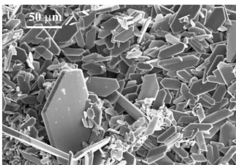
**Fig. 6** SEM image of electrodeposited thin films of (BEDT-TTF)[Ni(dcbdt)<sub>2</sub>].
