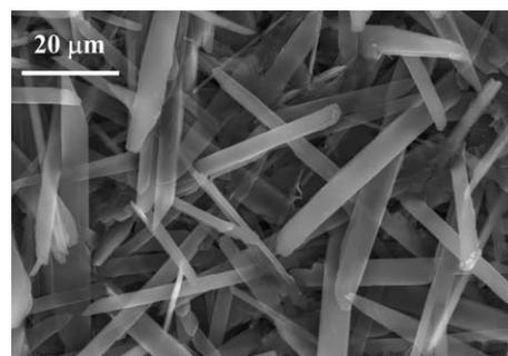
**Fig. 1** SEM image of the deposit of  $[(n\text{-C}_4\text{H}_9)_4\text{N}]_2[\text{Ni}(\text{dcbdt})_2]_5$ .
