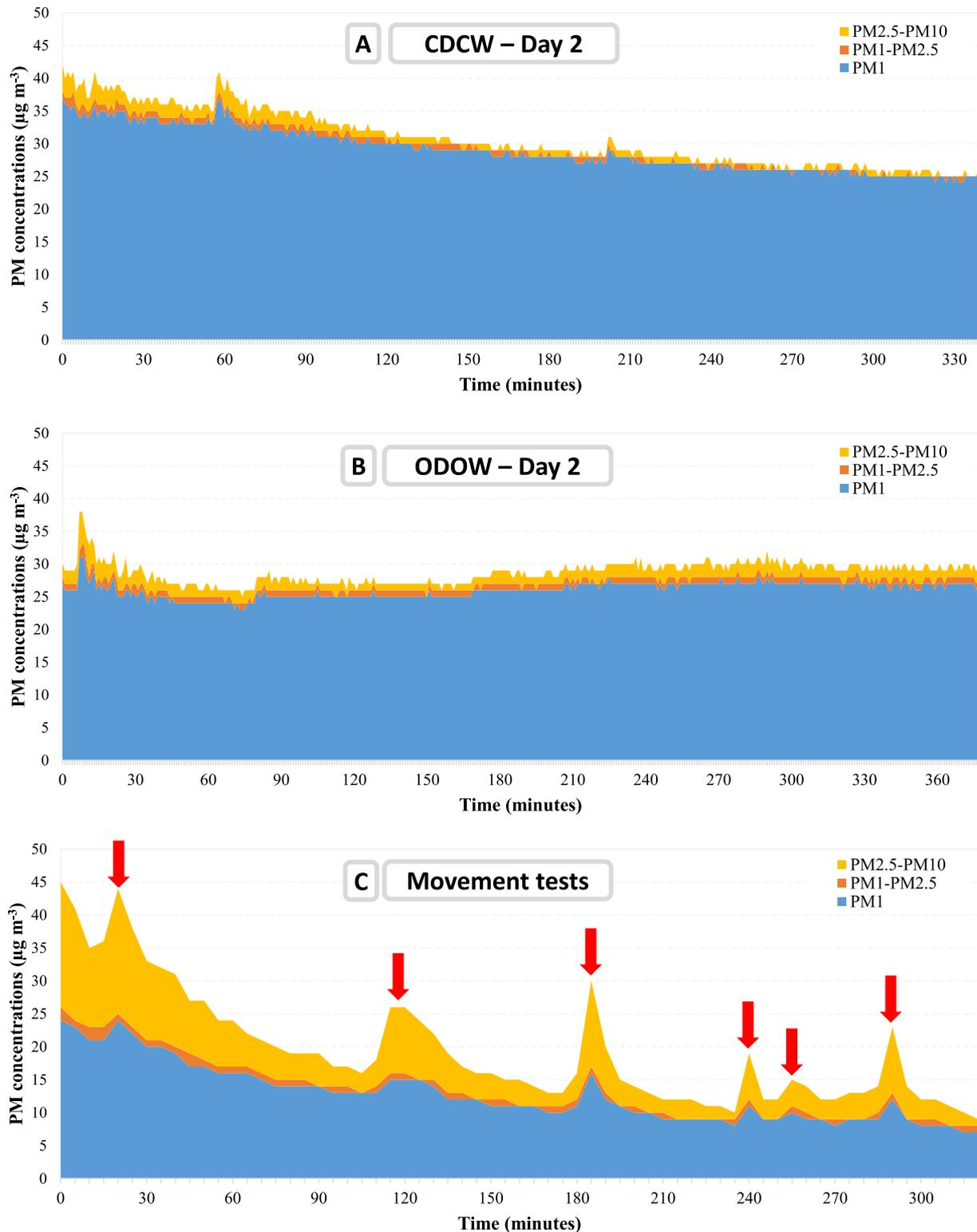
**Fig. 5.** Temporal variation of PM during sleeping: (A) Ventilation setting CDCW – day 2; (B) Ventilation setting ODOV – day 2 and (C) Movement tests during sleep with ventilation setting CDCW (red arrows indicates scheduled movements).
