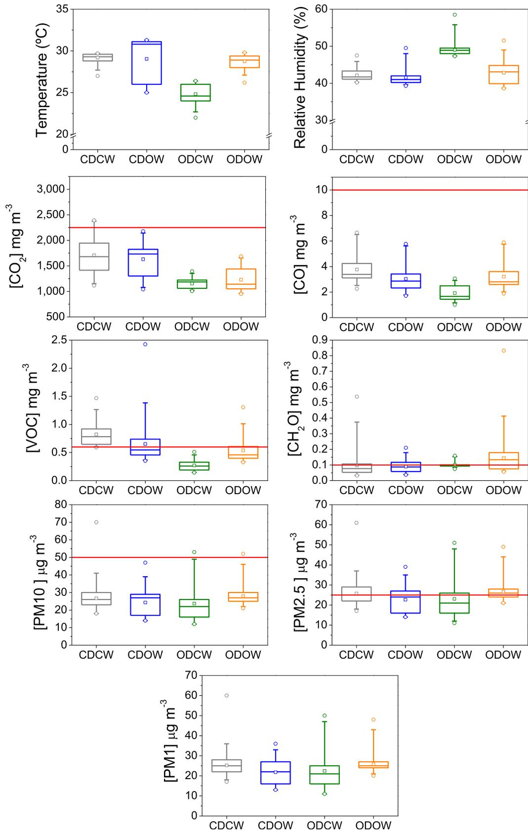
**Fig. 3.** Levels of indoor pollutants and comfort parameters during sleep under 4 different ventilation conditions (CDCW – closed door and closed window, CDOW – closed door and open window, ODCW – open door and closed window, ODOV – open door and open window). Red line represents the limit value defined by the Portuguese legislation (Ordinance no. 353-A/2013, 2013).
