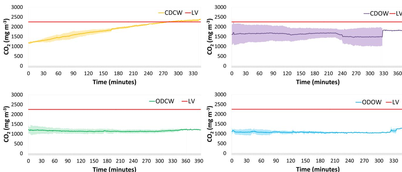
**Fig. 4.** Temporal variability of CO<sub>2</sub> (line – mean; light coloured area – standard deviation) during the sleeping period for the four studied ventilation settings: (top, left) CDCW, (top, right) CDOW, (bottom, left) ODCW and (bottom, right) ODOW. Red line represents the CO<sub>2</sub> limit value of 2250 mg m<sup>-3</sup> defined by the Portuguese legislation (Ordinance no. 353-A/2013, 2013).
