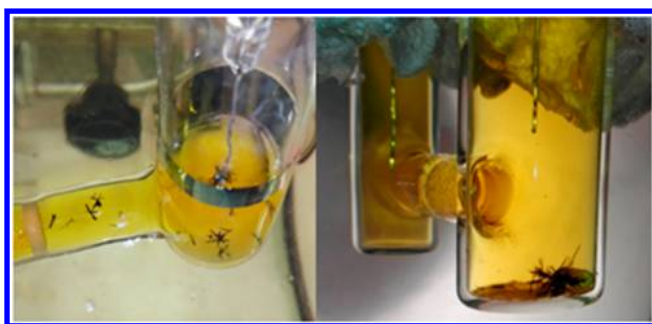
Figure 2. Dark crystals growing in the bottom of the electrocrystallization cell, over donor orange crystals which precipitate during the experiment.
