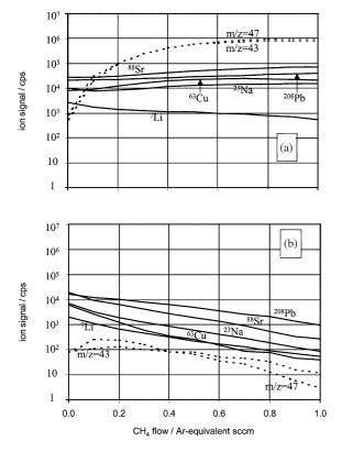
Fig. 27. Reaction profiles of analyte ions (solid lines) and unidentified ions produced within the cell (dashed lines) as a function of  $\mathrm{CH_4}$  reaction gas flow (1 Ar-equivalent sccm=0.52 sccm). (a) Without post-cell energy discrimination (quadrupole rod offset is -3 V, 2 V more negative than CRO). (b) With post-cell energy discrimination (quadrupole rod offset is +2 V, 3 V more positive than CRO).
