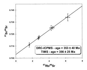
Fig. 36. Sr/Rb isochrone for an intrusive rock formation, obtained by dissolution and direct nebulization without element separation, using CH<sub>3</sub>F to convert the Sr<sup>+</sup> to SrF<sup>+</sup>, with Neon buffer to improve temporal homogenization. The derived age of the rock is in agreement with the TIMS result [161] and has comparable precision. (From Ref. [118] with permission of The Royal Society of Chemistry.)
