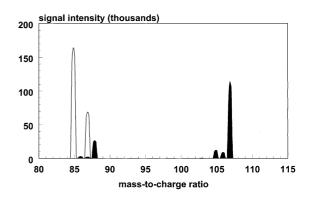
Fig. 35. Mass spectra for 50 ppb Rb and Sr, measured separately and overlaid to show the contributions of the isotopes to the combined spectrum, with CH<sub>3</sub>F as reaction gas. Sr<sup>+</sup> reacts to form SrF<sup>+</sup> (F is monoisotopic, so that the isotope ratio of SrF<sup>+</sup> reflects the isotope ratio of SrF<sup>+</sup>), and Rb<sup>+</sup> is unreactive. (From Ref. [118] with permission of The Royal Society of Chemistry.)
