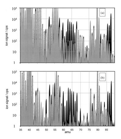
Fig. 28. Mass spectra for high purity water (grey) and a solution containing 1 ppb each of K, Ca, Cr, Mn, Fe, Ni, Cu, Zn, Se and Sr (black), with  $H_2$  as reaction gas at a flow of 0.4 Ar-equivalent sccm (0.28 sccm) and the cell operated with a wide transmission bandpass (RPa, RPq) = (0, 0.15). (a) Without post-cell energy discrimination (QRO = -3, CRO = -1). (b) With post-cell energy discrimination (QRO = +2, CRO = -1).
