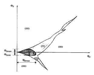
Fig. 14. Stability diagram for a hexapole for ions introduced at radial displacement  $r = 0.1r_0$ , obtained by theoretical modeling. Three regions of relative stability are shown: stable (I), partial stability (II) and unstable (III). (From Ref. [34] with permission from Elsevier Science.)
