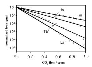
Fig. 6. Ion signals for lanthanide ions as a function of  $CO_2$  reaction gas flow (in true sccm). The steepest slope indicates the fastest reacting ion with the indicated gas.
