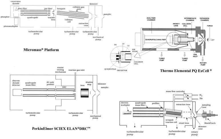
Fig. 4. Schematics of the four cell-based quadrupole analyzer instruments that are presently commercially available: the Micromass<sup>®</sup> Platform (figure courtesy Andrew Eaton), the Perkin Elmer SCIEX ELAN<sup>®</sup> DRC<sup>™</sup> (figure from the authors), the Thermo Elemental PQ ExCell<sup>®</sup> (figure courtesy Jonathan Batey) and the Agilent 7500c (figure courtesy Setsuo Muramoto).
