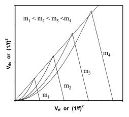
Fig. 11. Quadrupole stability diagrams as a function of ion mass, plotted in  $V_{\text{dc,rf}}/f^2$  space. Higher masses are stable at higher amplitude of the r.f. and DC and at lower operating frequency. The mass filter is usually operated by scanning the amplitudes of the voltages such that the tips of the stability boundaries are intersected.
