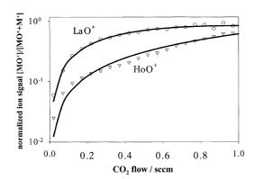
Fig. 8. Signals for the product ions of reactions of La and Ho with  $CO_2$  (see also Fig. 6). The more rapid increase of the  $LaO^+$  signal reflects the faster reaction of  $La^+$ . Further, the approach to unity of the normalization to the total  $(M^+ + MO^+)$  signal indicates that oxidation is the primary reaction channel for these ions.
