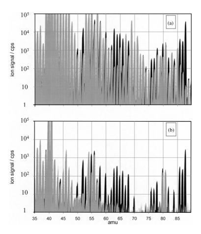
Fig. 29. Mass spectra for high purity water (grey) and a solution containing 1 ppb each of K, Ca, Cr, Mn, Fe, Ni, Cu, Zn, Se and Sr (black), with  $CH_4$  as reaction gas at a flow of 0.4 Ar-equivalent sccm (0.21 sccm) and the cell operated with a wide transmission bandpass (RPa, RPq) = (0, 0.15). (a) Without post-cell energy discrimination (QRO = -3, CRO = -1). (b) With post-cell energy discrimination (QRO = +2, CRO = -1).
