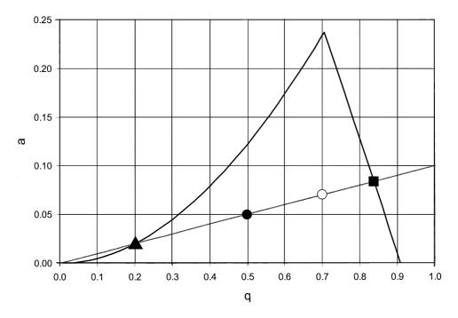
Fig. 30. Quadrupole stability diagram with hypothetical scan line. (▲) Denotes the high mass cut-off, and (■) denotes the low mass cut-off. The bandpass includes a lower mass range when operated at (●) than at (○), and this can affect the formation of secondary interferences if the precursor ion is included/excluded under these conditions.
