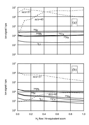
Fig. 26. Reaction profiles of analyte ions (solid lines) and unidentified ions produced within the cell (dashed lines) as a function of  $\rm H_2$  reaction gas flow (1 Ar-equivalent sccm=0.7 sccm). (a) Without post-cell energy discrimination (quadrupole rod offset is -3 V, 2 V more negative than CRO). (b) With post-cell energy discrimination (quadrupole rod offset is +2 V, 3 V more positive than CRO).
