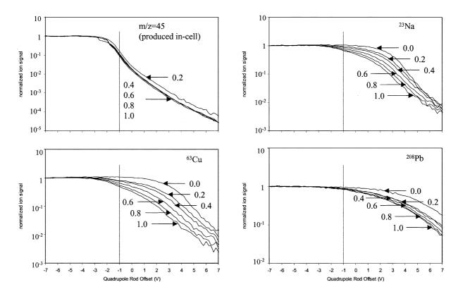
Fig. 24. Ion signals for several ions as a function of quadrupole rod offset potential for various  $H_2$  gas flows. The gas flow, in Arequivalent sccm (1 unit=0.7 sccm  $H_2$ ), is given beside the arrows. The CRO was -1.0 V (indicated by the grey vertical line). The ion at m/z=45 (not identified) is primarily produced within the cell. Ion energies tend towards the in-cell ion energy (near the CRO potential) at higher  $H_2$  flows and lower ion masses. Note that the vertical scales differ.
