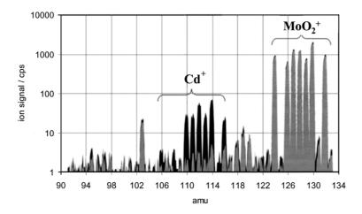
Fig. 39. Mass spectrum of a solution containing 10 ppb Mo with (black) and without (grey) 10 ppt Cd, obtained with  $O_2$  reaction gas (1.6 Ar-equivalent sccm=1.14 sccm), (RPa, RPq)=(0, 0.75). Oxidation of MoO<sup>+</sup> to MoO<sub>2</sub><sup>+</sup> relieves the interference of the monoxide ion on Cd<sup>+</sup>.
