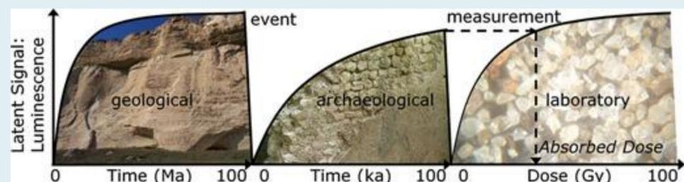
Dosimetric history of a mineral grain for luminescence dating. [4]
