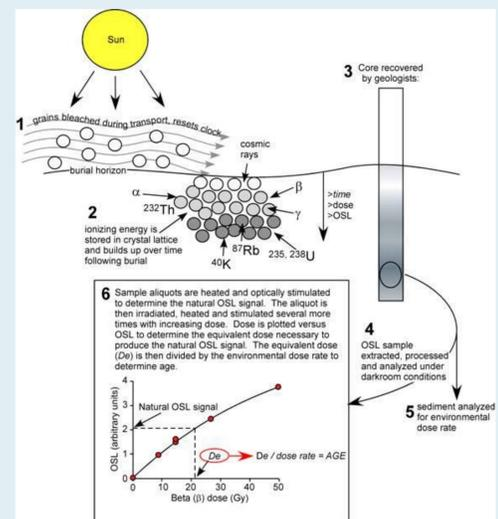
Generalized processes that produce the luminescence signal (steps 1 and 2), and the sampling and analytical procedure to determine the age of deposition (steps 3 through 6). [3]
