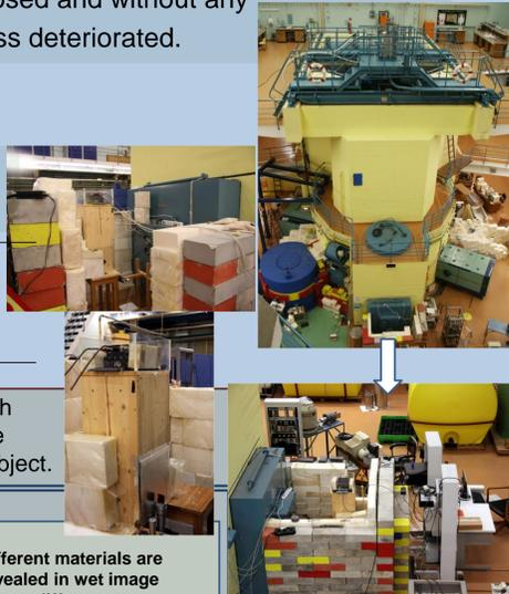
Advantages of NT: neutrons have a high interaction probability with hydrogen which allows to evaluate the degradation state of the tile and visualize the water and consolidants penetration inside the object.
