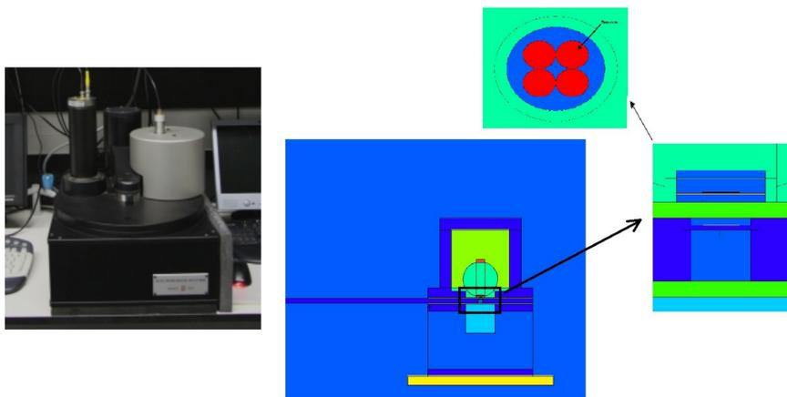
Figure 1: Geometric details of the Risø Reader as implemented in the MC Code.
