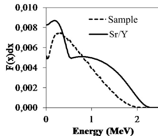
Figure 2: Normalized  $\beta$  particle energy distribution of Sr/Y and at the Quartz sample.
