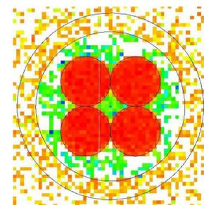
Figure 3: Energy deposition tallied around the Sr/Y source.
