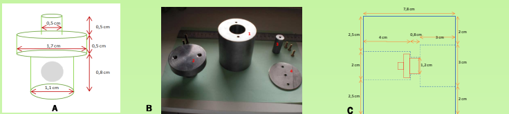
Figure 1. A - The ^{137}\text{Cs} source with the spherical shape (in grey) inside the acrylic covering. B - The several components of the irradiator. 1- Main body, 2-Removable cover, 3- Cylinder of lead, 4-Lid. C - The schematic design of the main body of the irradiator with the source.
