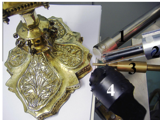
Fig. 1. Experimental setup at ITN, with the reliquary (CMAG 1194 Collection) placed in front of the external beam (3 mm distance) before the analysis; (1) X-ray detector with Mylar foil; (2) micro-camera; (3) beam exit nozzle with 100 nm \text{Si}_3\text{N}_4 window; (4) RBS detector with He flow.
