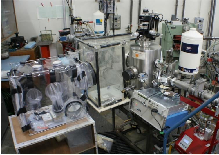
**Fig. 2** Experimental chamber dedicated to study large and contaminated materials with tritium and beryllium from fusion reactors
