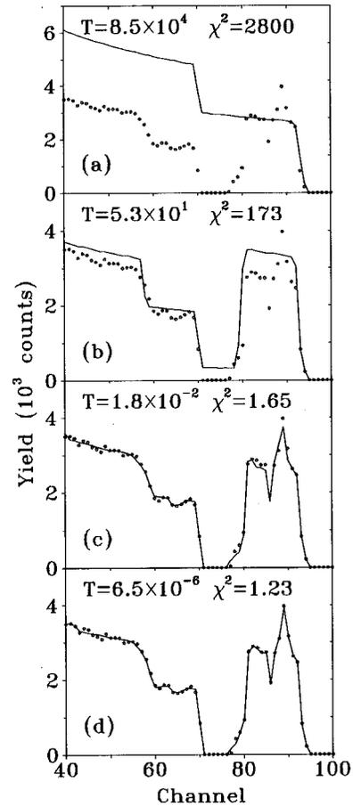
FIG. 2. Different steps of the fit, from (a) the initial guess to (d) the final result. The values of the control parameter  $T$  and  $\chi^2$  at each step are shown. On real data,  $\chi^2=1$  would mean that the fit is within the statistical error in all data points.
