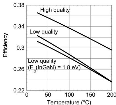
FIG. 8. Plot of the efficiencies of  $\text{InGaN}/\text{Si}$  two-junction solar cells as a function of cell temperature under 500 times concentration of the AM 1.5 global solar spectrum. The cell thicknesses were taken to be those that maximized the calculated efficiencies for each type of material (high or low quality).
