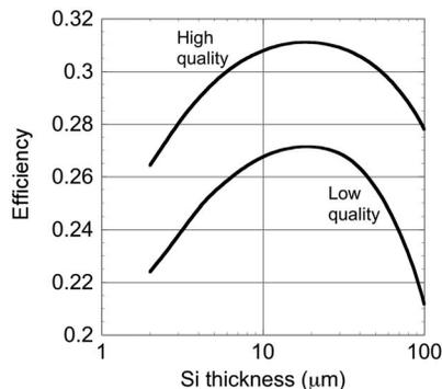
FIG. 5. Plot of the maximum efficiencies of InGaN/Si two-junction solar cells as a function of the physical thickness of the Si junction. The alloy composition of the InGaN junction was taken to be the one that maximizes the cell's efficiency, as shown in Fig. 4. The effective optical thickness of the Si junction was taken to be four times larger than the physical thickness.
