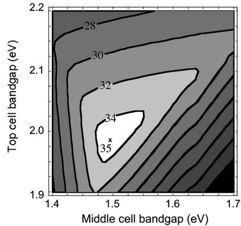
FIG. 9. Isoefficiency plot of an  $\text{InGaN}/\text{InGaN}/\text{Si}$  three-junction solar cell as a function of the bandgaps of the two  $\text{InGaN}$  junctions. The thickness of the  $\text{Si}$  junction is 20  $\mu\text{m}$ . The thicknesses of the  $\text{InGaN}$  junctions were taken to be those that maximized the short circuit currents of the corresponding one-junction  $\text{InGaN}$  solar cells.
