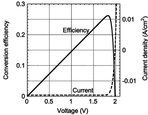
FIG. 7. Plot of the conversion efficiency (solid line) and current density (dashed line) vs operating voltage for a "low quality"  $\text{In}_{0.46}\text{Ga}_{0.54}\text{N}/\text{Si}$  two-junction solar cell.
