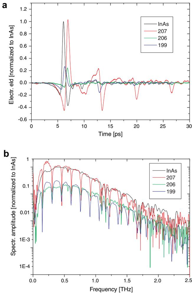
Fig. 2. Examples of InN emission during 800 nm excitation: (a) electric field amplitude, and (b) spectral amplitude.
