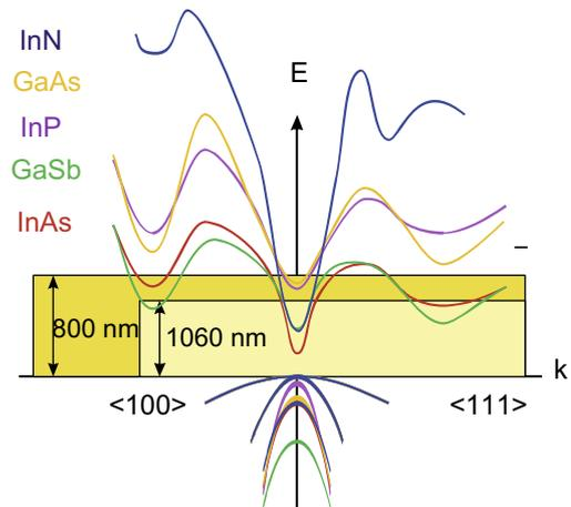
Fig. 6. Schematic of the energy bands for different THz emitting semiconductors in comparison to InN.
