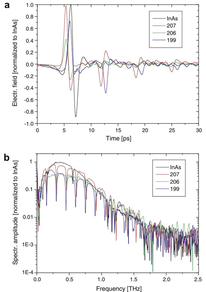
Fig. 3. Examples of InN emission during 1060 nm excitation: (a) electric field amplitude, and (b) spectral amplitude.
