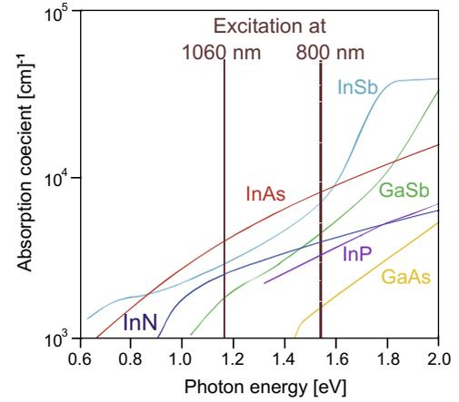
Fig. 5. Absorption coefficient for the semiconductors listed in Table 2; [30].
