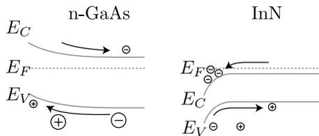
Fig. 4. Photo carrier separation in n-GaAs and InN due to surface band bending.
