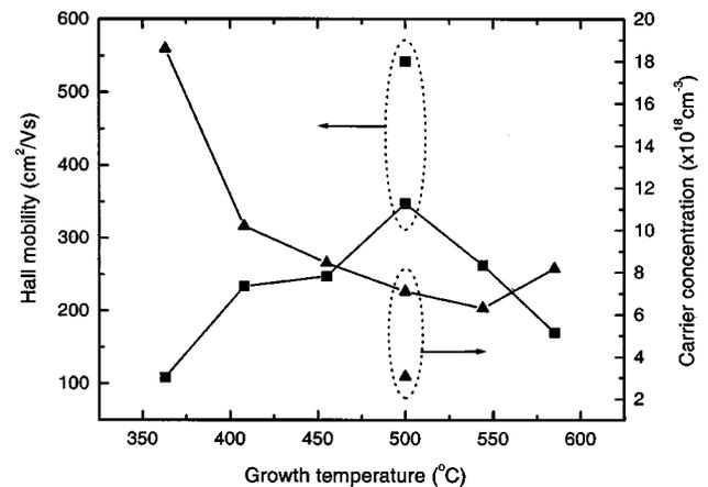
FIG. 3. Room-temperature Hall mobility and carrier concentration of the InN films as a function of substrate temperature. The separate points on the figure correspond to the electrical properties of a special sample grown on 2 in. sapphire with  $0.2 \mu\text{m}$  thickness.
