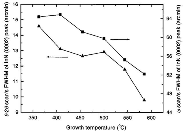
FIG. 2. Substrate temperature dependence of the FWHM of the InN (0002) peak in the XRD  $\theta$ - $2\theta$  scan and  $\omega$  scan.
