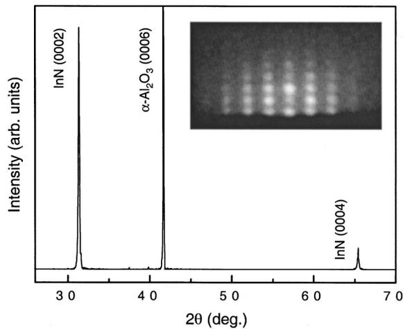
FIG. 1. Typical  $\theta$ - $2\theta$  XRD profile of the grown InN by MEE. The inset is a typical spotty RHEED pattern observed along the  $[10\bar{1}0]$  azimuth during growth.
