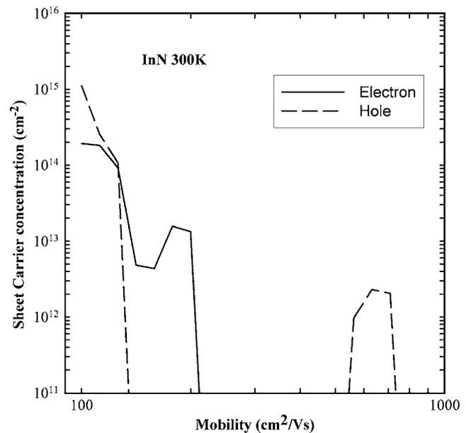
FIG. 2. QMSA spectrum of the  $3 \times 10^{20} \text{ cm}^{-3}$  Mg-doped film at 300 K showing light hole, heavy hole, and electron conduction.
