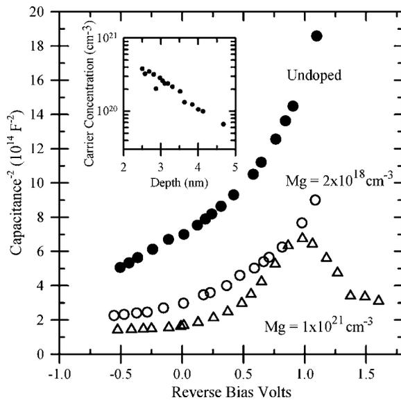
FIG. 1. Electrolytic capacitance-voltage measurements on unintentionally and Mg-doped InN films. Inset: concentration, due primarily to the near surface accumulation layer, is  $1.8 \times 10^{13} \text{ cm}^{-2}$ , close to the  $1.6 \times 10^{13} \text{ cm}^{-2}$  result obtained by others (Ref. 4).
