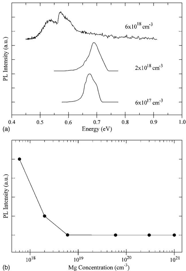
FIG. 3. (a) Photoluminescence signals (488 nm argon laser line, InSb detector) from three lightly Mg-doped InN films. (b) The 0.68 eV peak intensity measured from InN films as a function of Mg concentration.
