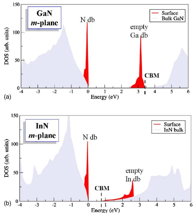
FIG. 4. (Color online) Density of states for the stable surface structures found for moderate Ga(In)/N ratios on the nonpolar GaN(InN) ( $1\bar{1}00$ ) surfaces. (a) GaN dimer structure; (b) InN dimer structure.
