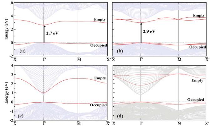
FIG. 3. (Color online) Electronic band structures of the (a) GaN dimer ( $1\bar{1}00$ ); (b) GaN dimers ( $11\bar{2}0$ ); (c) InN dimer ( $1\bar{1}00$ ); and (d) InN dimer ( $11\bar{2}0$ ) reconstructed surfaces. Gray lines indicate the projected bulk band structure. The zero of energy is set at the bulk VBM. Relevant energy differences between the VBM and surface states (in red) are indicated by arrows.
