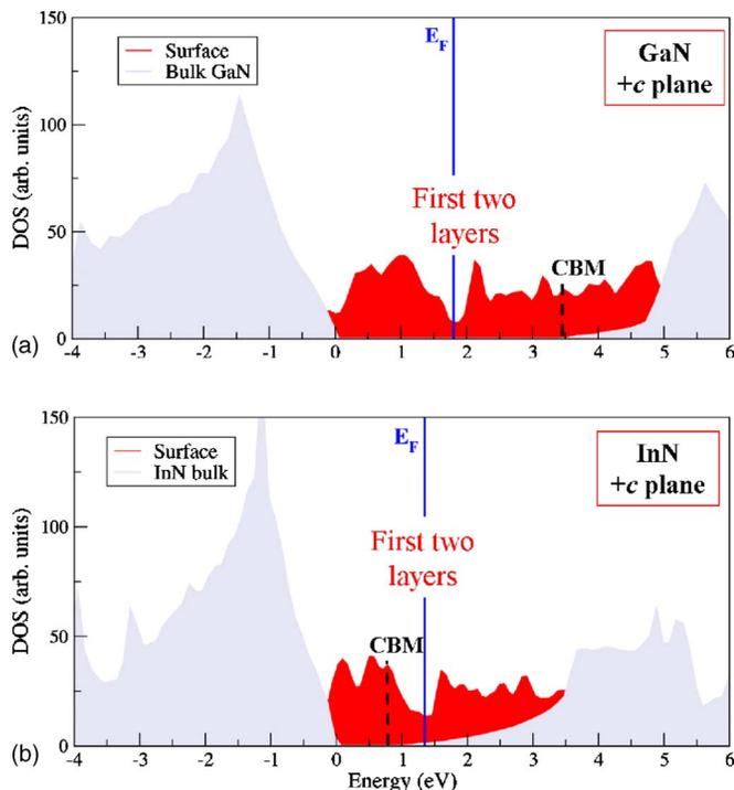
FIG. 5. (Color online) Density of states for the stable surface structure (laterally contracted bilayer) found under Ga(In)-rich conditions on the polar (0001) surfaces of (a) GaN and (b) InN.
