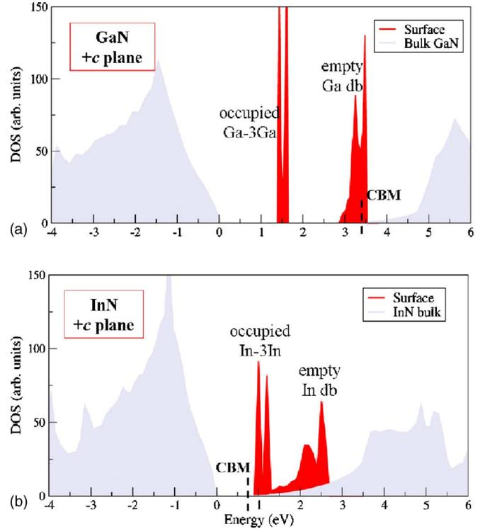
FIG. 2. (Color online) Density of states for the stable surface structures found for moderate Ga(In)/N ratios on the polar  $\text{GaN}(\text{InN})$  (0001) surfaces. (a)  $\text{GaN}$ :  $2 \times 2$   $\text{Ga}_{T4}$  (0001) structure; (b)  $\text{InN}$ :  $2 \times 2$   $\text{In}_{T4}$  (0001) structure.
