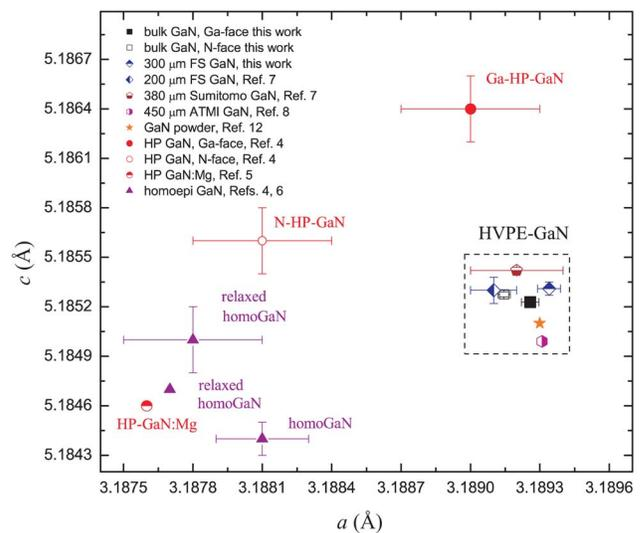
FIG. 2. (Color online) Lattice parameters  $a$  and  $c$  for bulk and freestanding GaN fabricated by HVPE, HP bulk GaN, and homoepitaxial GaN layer.
