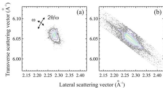
FIG. 1. (Color online) Reciprocal space maps around the GaN 105 reciprocal lattice point of (a) the 2-mm-thick HVPE bulk GaN and (b) 300- $\mu\text{m}$ -thick HVPE GaN freestanding separated by laser lift-off from the substrate. The RSMs are normalized to the maximum intensity and the same seven contour levels (from 0.0001 to 1) equidistant in log scale are used in (a) and (b).
