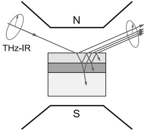
Fig. 1. The principle of an optical Hall-effect measurement. Magneto-optical generalized ellipsometry (MOGE) at infrared and THz wavelengths is used for precise measurement of the optical Hall effect in layered semiconductor heterostructures. The experimental MOGE setup and data analysis are detailed in Ref. 13.
