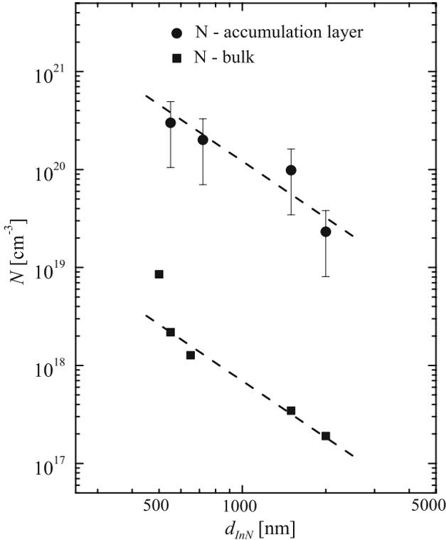
Fig. 5. InN bulk and surface electron accumulation densities as a function of the layer thickness. Both the bulk and the surface electron accumulation density follow the same power law ( $N \sim d_{\text{InN}}^{-1.92}$ ) in the investigated thickness region.
