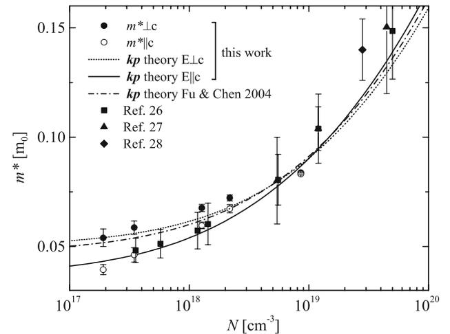
Fig. 4. Effective mass parameters of hexagonal InN for polarization parallel and perpendicular to the  $c$ -axis obtained from MOGE analysis. Data from previous reports and  $kp$  calculations are included for comparison.<sup>26-28</sup>
