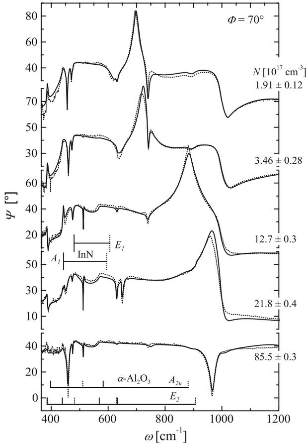
Fig. 2. Field-free ( $\mu_0 H = 0$ ) experimental (dotted) and best-model calculated (solid lines) IRSE  $\Psi$  spectra from InN thin films deposited on  $c$ -plane sapphire with varying thickness and free electron density.
