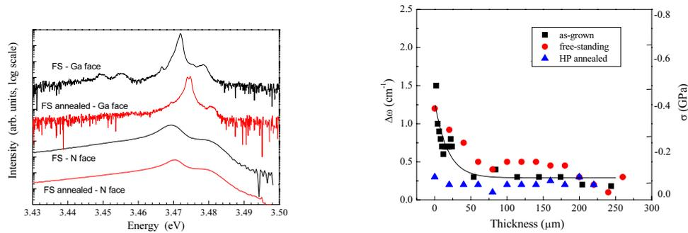
**Fig. 2** (left) Low temperature PL spectra of FS self-separated films before and after the HP annealing at 1450 °C taken from both the Ga and N faces.
