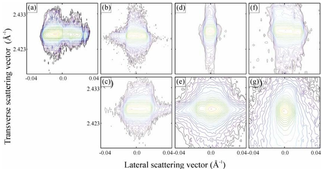
**Fig. 1** Reciprocal space maps around the GaN 0002 reciprocal space point of a 270  $\mu\text{m}$ -thick HVPE-GaN film: (a) residing on sapphire; (b,c) FS self-separated; (d,e) FS after laser-lift off separation; (f,g) FS after LLO and polishing taken from the Ga face (a,b,d,f) and N face (c,e,g) of the free-standing films.
