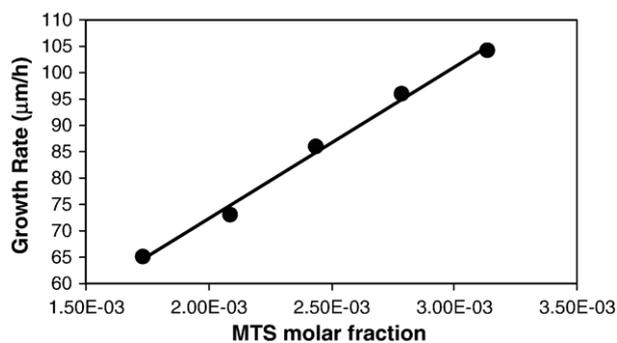
Fig. 1. Growth rate of 4H-SiC epitaxial layers for various flows of MTS. All layers are grown at  $1600^\circ\text{C}$  using only MTS as precursor; only the flow of MTS into the reactor is changed between the runs.
