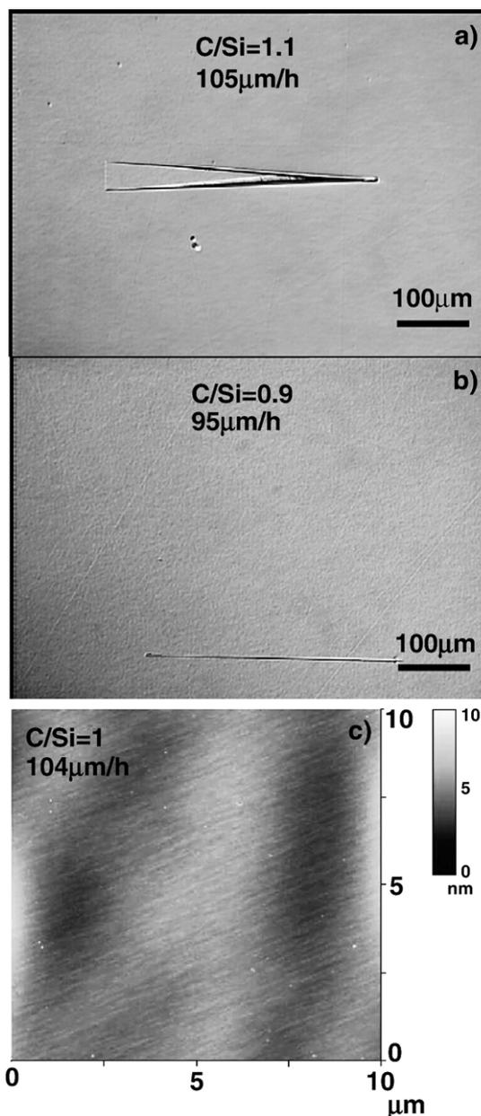
Fig. 2. The morphology of the epitaxial layers illustrated by Nomarski microscope images showing the morphology and epi-defect shape of a) a  $52 \mu\text{m}$  thick epilayer grown with  $C/Si = 1.1$  and b) a  $48 \mu\text{m}$  thick epilayer grown with  $C/Si = 0.9$ , in c) a  $10 \times 10 \mu\text{m}^2$  AFM image of a  $52 \mu\text{m}$  thick epilayer grown with  $C/Si = 1$ ; the RMS value is  $7 \text{ \AA}$ .
