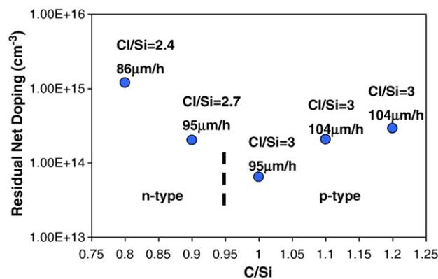
Fig. 5. The residual net doping for various C/Si ratios. Note that the growth rate and C/Si ratio are not the same for all runs, as indicated by the inserts in the plot. The dashed vertical line in the plot shows which epilayers are n- and p-type.
