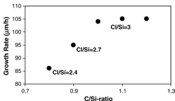
Fig. 4. Growth rate of 4H-SiC epitaxial layers for various C/Si ratios. The total amount of Si into the reactor is constant for all the runs, the changing C/Si ratio is indicated in the plot.
