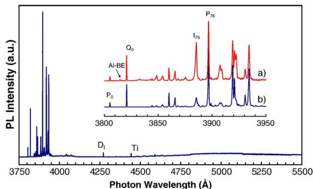
Fig. 3. LTPL spectra recorded from a sample grown with C/Si=0.9 and a growth rate of 95  $\mu\text{m}/\text{h}$ . The inset shows the near-band gap emission for a) the same sample and b) a sample with C/Si=1.2 grown at 105  $\mu\text{m}/\text{h}$ .
