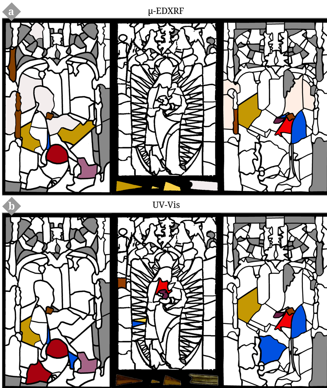
Fig. 6 Classification of glass colours (constituent fragments) based on a \mu -EDXRF and b UV-vis results—false colour maps. Gray areas represent modern glass insets (probably introduced during the nineteenth century)
