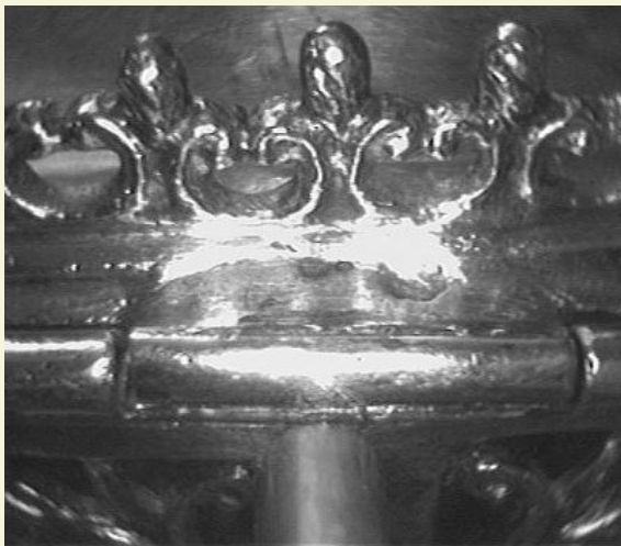
Figure 9. a) Elemental distribution of Ag, Cu, Hg and Au; b) View of the exit nozzle and the object to be analyzed (the fastener of the reliquary (GMAG 1194)).
