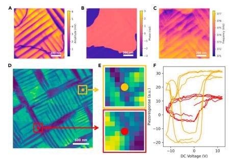
Figure 1. Band excitation piezoresponse force microscopy (BEPFM) and spectroscopy (BEPS) results of model sample PbTiO<sub>3</sub> (A-C) BEPFM amplitude, phase, and frequency images showing ferroelectric and ferroelastic domain structures in PTO thin film.
