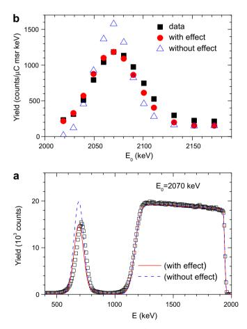
Fig. 2. (a) RBS spectrum of a Mylar 1  $\mu$ m/Ni 4.2  $\mu$ m sample, collected at  $E_0 = 2070$  keV. (b) Integrated C yield as a function of beam energy. The data and calculated values with and without the resonance effect are shown.
