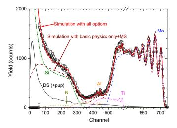
Fig. 1. RBS spectrum of a Si/ $(Ti_{0.4}Al_{0.6}N 25.2 \text{ Å} /Mo 14.9 \text{ Å})_{\times 10}$  multilayer measured at 5° grazing angle. A full simulation including double scattering (DS), pulse pile-up (pup), roughness and an improved low energy yield calculation is shown. The calculated partial signals of the elements are shown. A simulation including only basic physics (but with the correct energy straggling) is also shown for comparison.
