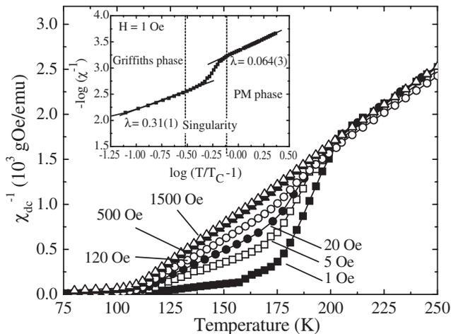
FIG. 1. Temperature dependence of  $\chi^{-1}$  as a function of magnetic field, measured on heating. The inset shows fits at 1 Oe in the Griffiths and PM phases, respectively.
