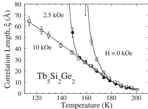
FIG. 3. Temperature and field dependence of  $\xi$  calculated from the Lorentzian fits of the SANS spectra.
