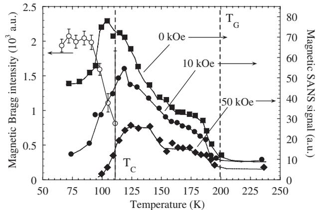
FIG. 2. Temperature dependence of the magnetic SANS intensity collected in D16 at  $q = 0.1 \text{ \AA}^{-1}$  in different magnetic fields (filled symbols), in comparison with the intensity of a magnetic Bragg peak extracted from Ref. [19] (empty symbols).
