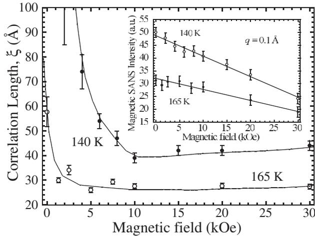
FIG. 4. Magnetic-field dependence of  $\xi$  at  $T = 140$  and  $165$  K. The inset displays the isothermal dependence of the SANS intensity as a function of the magnetic field at  $q = 0.1 \text{ \AA}^{-1}$  for the same temperatures.
