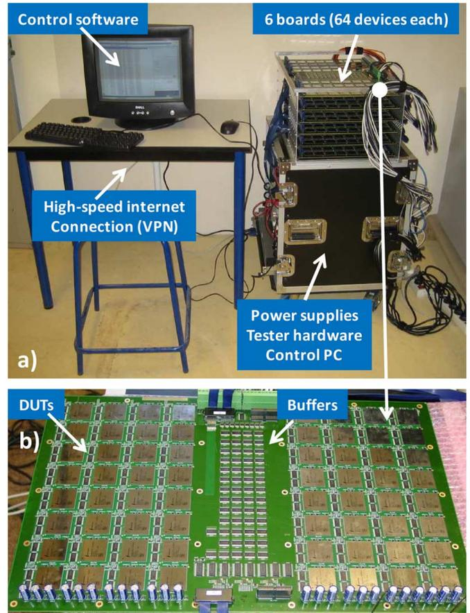
Fig. 2. a) General view of the SRAM automatic test equipment (here photographed on the ASTEP platform) and b) detail of one motherboard. The system is designed to test 384 chips dispatched on 6 motherboards. Chips (directly connected on motherboards) are horizontally oriented during the test. The system deployed at LSM is strictly identical for both hardware and software aspects.
