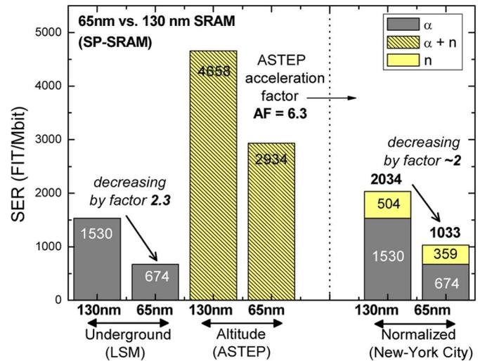
Fig. 8. Synthesis of experimental real-time SER values obtained for both 130 nm and 65 nm SP-SRAM from altitude and underground experiments and normalization of the SER at the reference flux of New-York City (sea-level) [4] taking into account i) the alpha contribution for the altitude test (fixed to the value measured at LSM) and ii) the ASTEP acceleration factor  $AF = 6.3$  for the neutron flux in altitude (experimentally measured using the Plateau de Bure Neutron Monitor).
