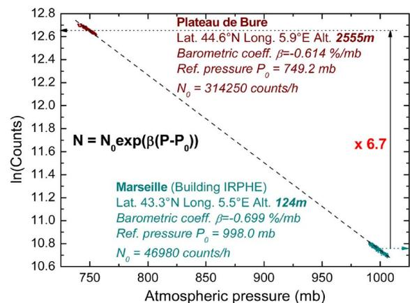
Fig. 4. Experimental determination of the ASTEP acceleration factor (AF) from the barometric response of the neutron monitor successively installed in Marseille (2007–2008) and on the Plateau de Bure since July 2008. Experimental clouds correspond to one month recording (one point per hour).
