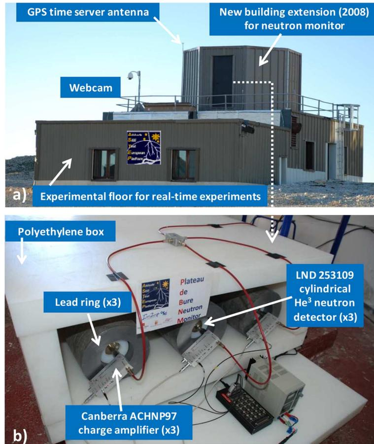
Fig. 3. a) External view ASTEP building showing the new extension (first floor) designed to host the Plateau de Bure Neutron Monitor (PdBNM). b) View of the extremities of the cylindrical neutron detector tubes connected to the charge amplifiers and to the acquisition module (electronic counters).
