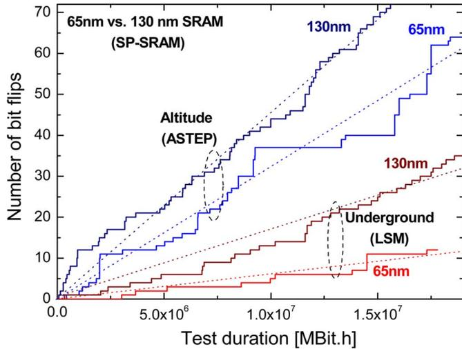
Fig. 7. Cumulative total fails versus test duration for both 130 nm and 65 nm SP-SRAMs detected in altitude and underground. Test has been conducted under nominal conditions for both technologies:  $V_{DD} = 1.2$  V, room temperature, standard checkerboard test pattern. For 130 nm data, experiment periods are [March 31, 2006–November 6, 2006] for the altitude test and [October 16, 2007–November 24, 2008] for the underground test.
