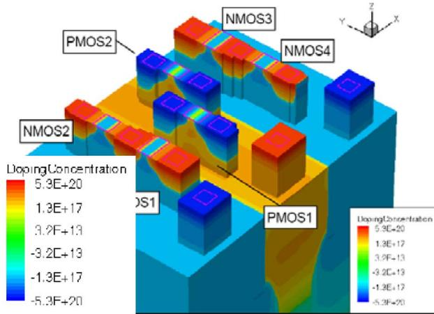
Fig. 1. Full 3-D structure of the bulk 65 nm SP-SRAM (6 transistors, bit cell area of  $0.525 \mu\text{m}^2$ ). STI structures have been removed for better showing Silicon regions below transistor active area. The simulation domain contains more than 300,000 mesh elements.
