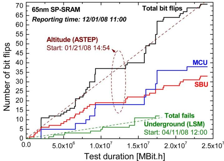
Fig. 5. Cumulative total fails, SBU and MCU flips versus test duration for the 65 nm SP-SRAM during both altitude and underground experiments. Test has been conducted under nominal conditions:  $V_{DD} = 1.2$  V, room temperature, standard checkerboard test pattern.
