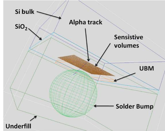
Fig. 3. Simulated geometrical structure generated by MC-ORACLE of a 65 nm technology node. As an indication of the scale, the sphere has diameter of 100  $\mu\text{m}$ .
