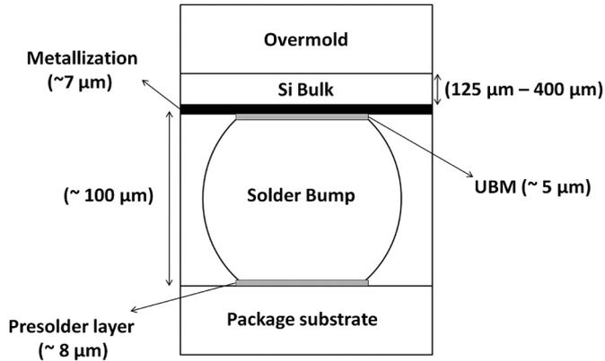
Fig. 1. Cross-sectional views of simplified flip chip device. (Not to scale).
