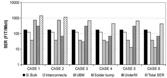
Fig. 4. Contribution to SER of different materials in a 65 nm flip chip device with different purity grades.
