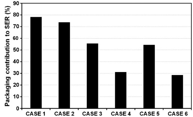
Fig. 5. Packaging contribution to alpha-SER in a 65 nm flip chip device in different cases.
