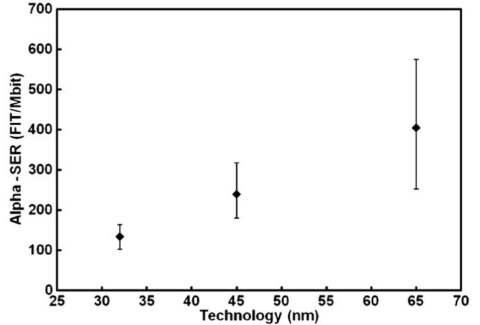
Fig. 6. SER induced by alpha particles for the 65, 45, and 32 nm technologies.
