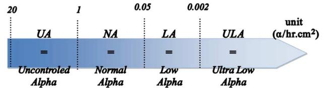
Fig. 2. Material classification according to the alpha emission rate.
