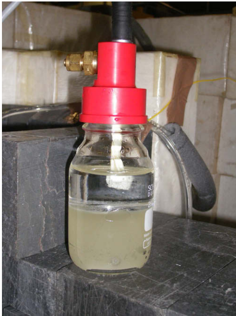
Fig. 3. Completed 150 ml CF 3 I detector prototype, with new capping. Note the encapsulated microphone in the glycerin layer.
