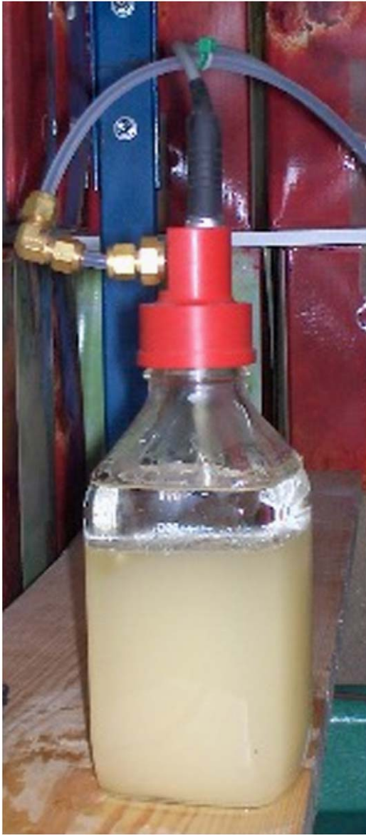
Fig. 1. SIMPLE detector and its instrumented cap, showing the microphone interface (vertical) and pressure couple (horizontal).
