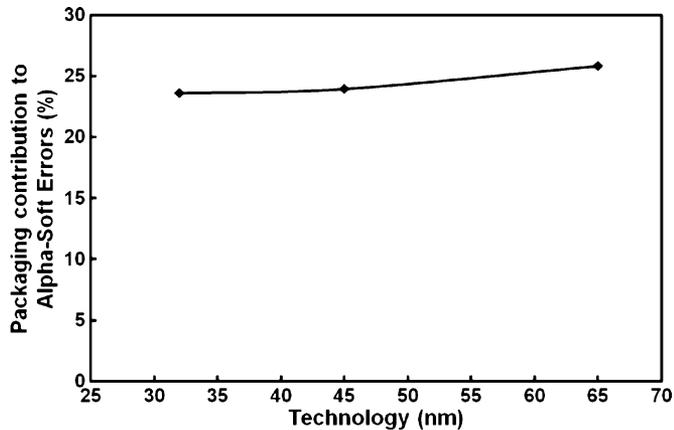
Fig. 7. Packaging contribution to SER for the 65, 45, and 32 nm technologies.
