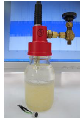
Fig. 1. A Sm-doped 150 ml SDD equipped with microphone and valve for pressurisation. The raw acoustic signal is displayed in the background. A discard microphone is shown in front of the detector.
