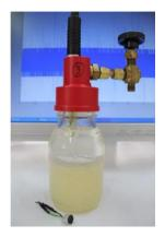
**Fig. 1.** A Sm-doped 150 ml SDD equipped with microphone and valve for pressurisation. The raw acoustic signal is displayed in the background. A discard microphone is shown in front of the detector.
