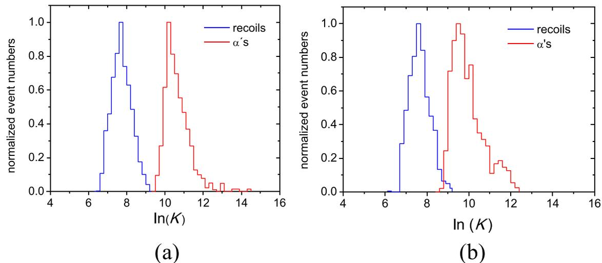
Fig. 2. Recoil- and  $\alpha$ -induced event power distributions for (a) neutron-then- $\alpha$  and (b)  $\alpha$ -then- neutron irradiations.
