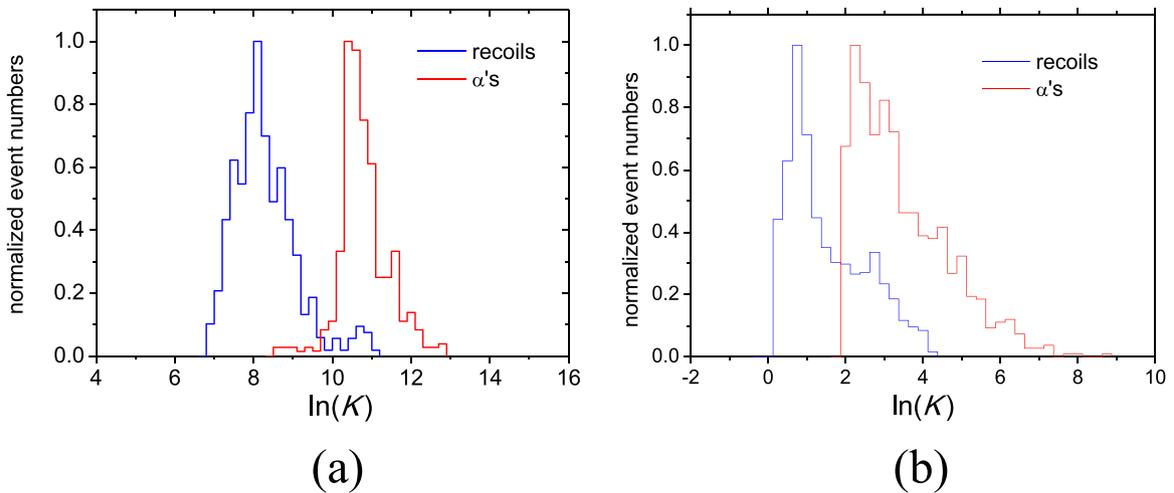
Fig. 5. (a) Spectra of recoil- and  $\alpha$ -induced event power distributions:  $C_4F_{10}$  SED at 27 °C/1 bar, with stiffer gel and  $\langle r \rangle \sim 23 \mu\text{m}$ ; (b)  $C_2ClF_5$  SED at 9 °C/1 bar,  $\langle r \rangle \sim 5.5 \mu\text{m}$ .
