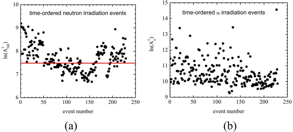
**Fig. 12.** Typical scatter plot of the first 230 recorded event amplitudes in neutron irradiation (a) and  $\alpha$  irradiation (b) of a SED, indicating the exposure-dependent populating of the eventual recoil distribution.
