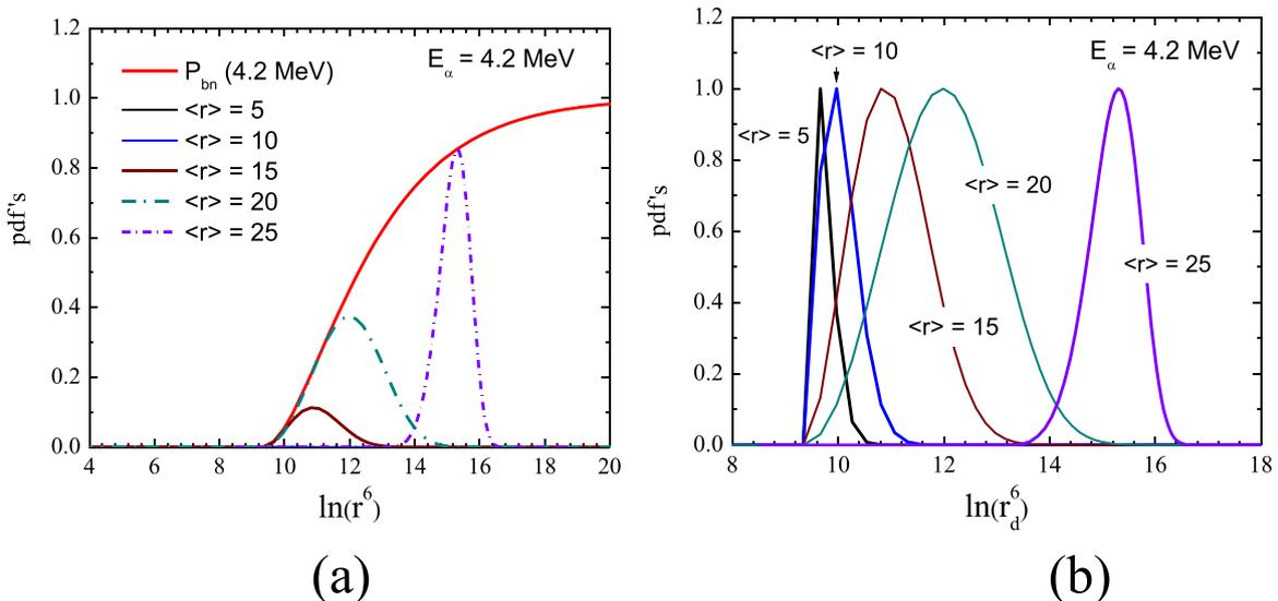
**Fig. 14.** (a) convolution of the bubble nucleation efficiency with Gaussian droplet size distributions of  $\langle r_d \rangle = 5 \pm 3, 10 \pm 3, 15 \pm 5, 20 \pm 7$  and  $25 \pm 8 \mu\text{m}$  and  $E_\alpha = 4.2 \text{ MeV}$ ; (b) same as (a) but with the simulated response now normalized.
