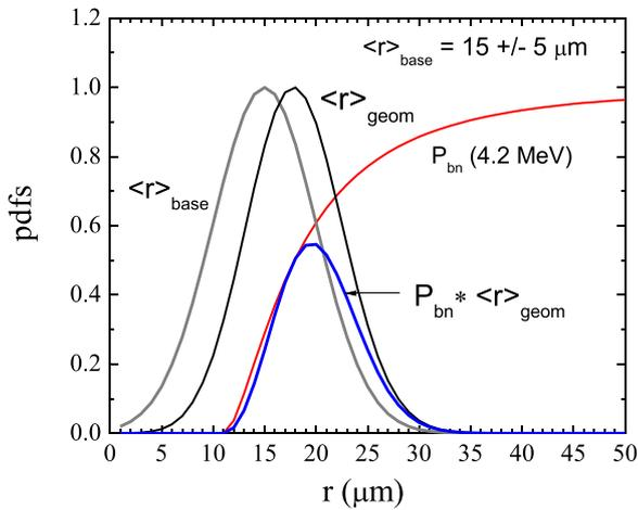
**Fig. 13.** Model interaction of a Gaussian droplet size distribution of  $\langle r \rangle = 15 \pm 5 \mu\text{m}$  with 4.2 MeV  $\alpha$ 's ( $p_c = 11 \mu\text{m}$ ).
