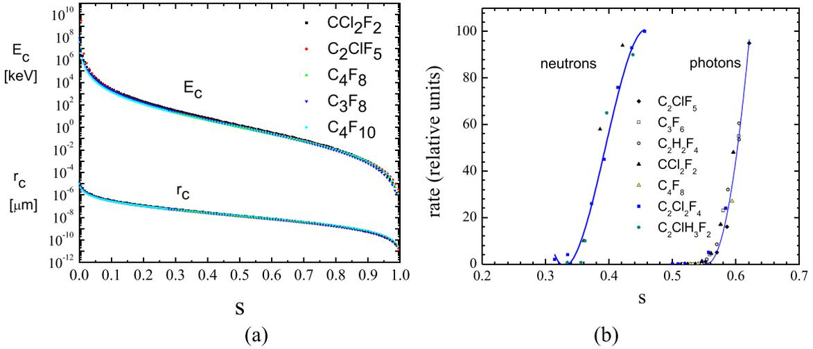
**Fig. 1.** (a) Universal behavior of  $E_c$  and  $r_c$  in terms of  $s$ ; (b)  $\gamma$  and neutron irradiation responses of various superheated liquids, which in  $s$  fall on single curves (adapted from Ref. [21]).
