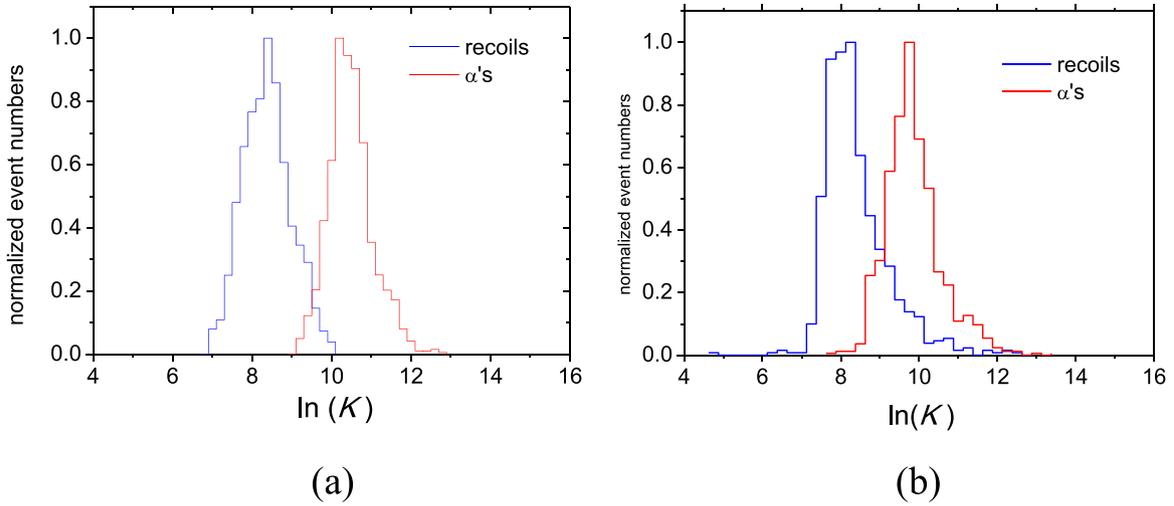
Fig. 3. Recoil- and  $\alpha$ -induced event power distributions as in Fig. 2: big droplet distribution.
