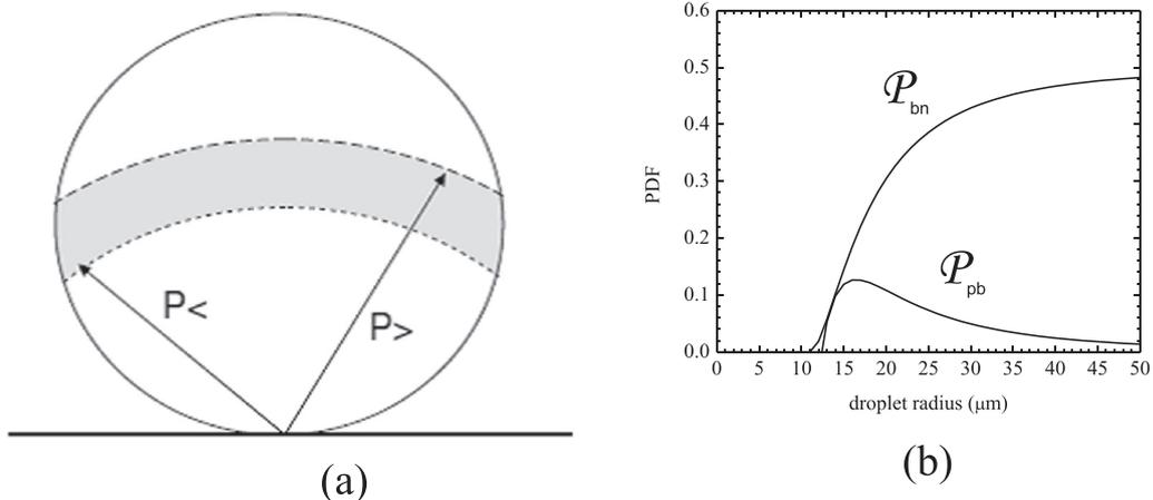
**Fig. 11.** (a) Scenario of the “surface emission” model: only  $\alpha$  particles originating from the droplet surface emitted into the shaded spherical volume may contribute; (b) variation of  $P_{\text{bn}}$  and  $P_{\text{pb}}$  with droplet radius for a Gaussian  $\langle r \rangle = 15 \pm 5 \mu\text{m}$  distribution.
