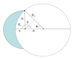
Figure 3. schematic view of the surface-emitted  $\alpha$  - droplet interaction; the  $\alpha$ 's must enter the shaded region of the droplet to provoke a bubble nucleation.
