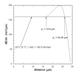
Figure 1. SRIM-computed 4.20 MeV  $\alpha$  Bragg curve in C<sub>2</sub>ClF<sub>5</sub> at 5 °C and ambient pressure. The intersection with the LET<sub>c</sub> (161 keV/µm) gives  $p_{<}$  (16.8 µm) and  $p_{>}$  (26.08 µm), respectively.
