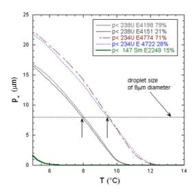
Figure 2. Variation of p < with temperature in  $C_2ClF_5$  required for bubble creation by isotopes of U and Sm with alpha's of energy E and % isotopic abundance.
