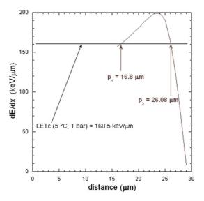
Figure 1. SRIM-computed 4.20 MeV alpha Bragg curve in  $C_2ClF_5$  at 5°C and ambient pressure. The intersection with the LET<sub>c</sub> (161 keV/ $\mu$ m) gives  $p_<$  (16.8  $\mu$ m) and  $p_>$  (26.08  $\mu$ m), respectively.
