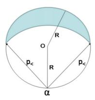
Figure 3. Schematic view of the surface-emitted alphadroplet interaction of center O; the alpha's must enter the shaded region of the droplet of radius *R* to provoke a bubble nucleation.
