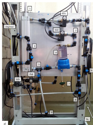
Fig. 3. Real picture of the automaton's blue line, where the piston goes from 2 to 8 bar. The N^2 gas used to compress the piston gets in the system through the tube on the right, straight up to EV1. This EV is the one controlling the amount of N^2 used to compress the blue piston and EV2 releases the N^2 when the chamber is de-compressing. The tube on the upper left corner is the one going straight to the chamber to apply the pressure changes made by both pistons. EV3 applies the pressure changes made by the blue piston and EV6 applies the ones made by the green piston. Caption: 1- blue piston, 2- L-connector (elbow), 3- Y-connector, 4- glycerine reservoir, 5- T-connector, 6- manual valve, 7- purge, 8- blanking plug, 9-cap.
