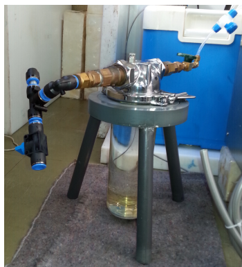
Fig. 2. Chamber on a tripod, with all the connections of the cap assembled. The yellow tonality observed, especially in lower part of the chamber's body, is due to the gel covering the chamber walls and bottom.
