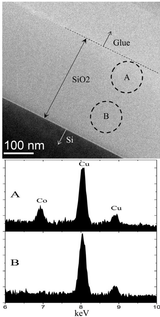
**Figure 2.** Bright field XTEM image of the Co implanted AAO/SiO<sub>2</sub>/Si sample with EDX spectra taken at different depths A and B. Region A is near the surface.
