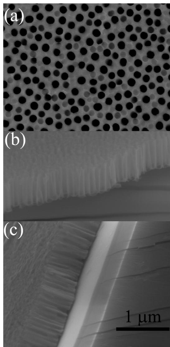
**Figure 1.** (a) Top view and (b), (c) side views of the AAO/SiO<sub>2</sub>/Si structure.
