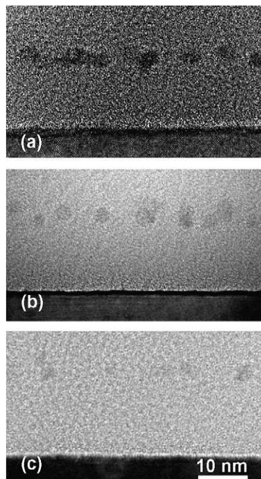
Fig. 1. Cross-sectional HREM image of: (a) sample B, (b) sample C. (c) Z-contrast STEM of sample D. Underfocus/overfocus conditions were selected to increase the visibility contrast of the nanoparticles.
