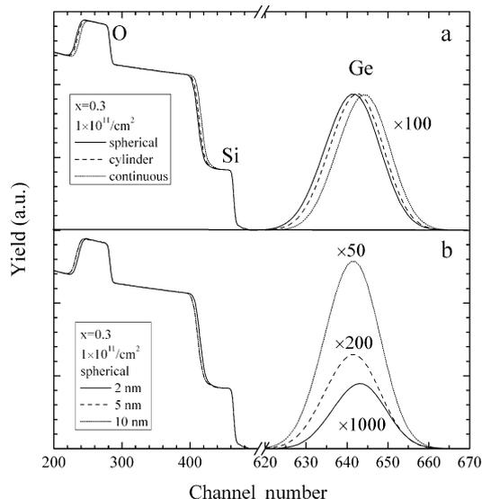
Fig. 2. Comparison of simulated RBS spectra assuming the existence (a) of spherical and cylindrical SiGe nanoparticles or a continuous SiGe layer embedded in SiO<sub>2</sub> and (b) of spherical SiGe nanoparticles with different diameters.
