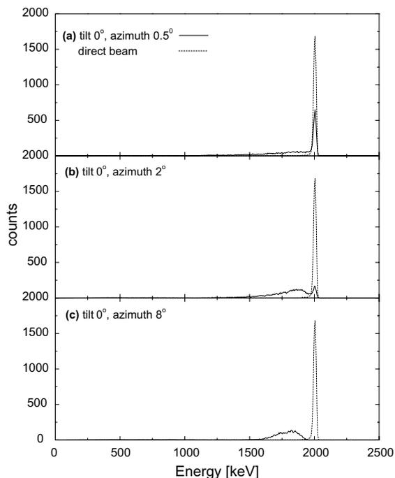
Fig. 3. Energy spectrum of transmitted beam through the sample A30 at three different orientations. The tilt and azimuth angle are measured from the initial position of the target wheel, nearly perpendicular to the beam. The width of the transmission peak ( $\sim 20$  keV) is comparable with the detector resolution.
