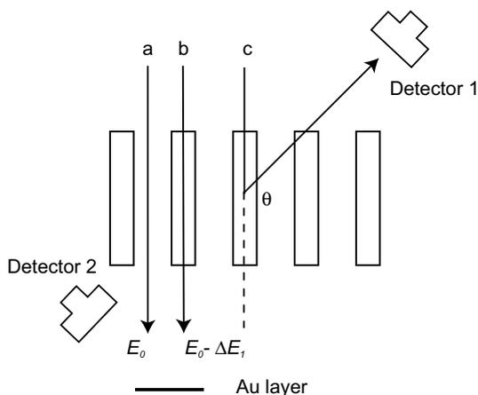
Fig. 9. Ion transmission through pores (a), solid material (b) and backscattering (c) at the aligned orientation of an ideal sample.
