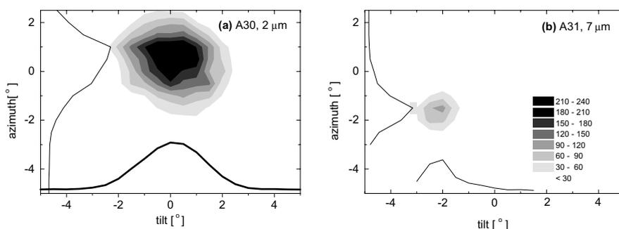
Fig. 4. Angular scans of the transmission through the pores for the 2  $\mu\text{m}$  thick sample A30 (a) and the 7  $\mu\text{m}$  thick sample A31 (b). Both angles were measured from the zero position of the target holder set perpendicular to the incident beam. The solid lines are projections of the peak on the tilt and azimuth axes in arbitrary units.
