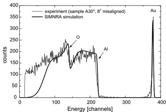
Fig. 11. Experimental and simulated RBS spectrum for the sample A30\* tilted  $8^\circ$  from the aligned direction. The simulation was performed by the SIMNRA code. The effective atomic surface density with an average value of  $55 \times 10^{17}$  atoms/cm<sup>2</sup> and FWHM of  $30 \times 10^{17}$  was assumed. A better agreement was achieved for  $\text{AlO}_2$  rather than  $\text{Al}_2\text{O}_3$  sample composition.
