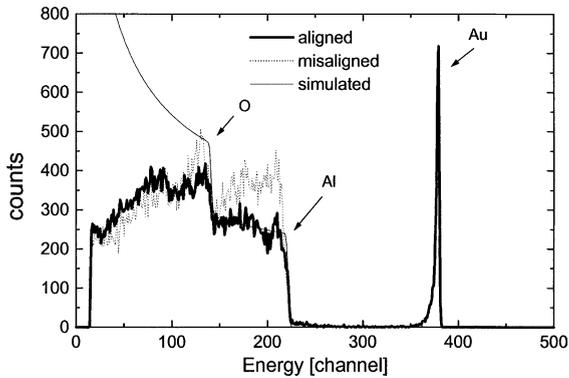
Fig. 7. RBS spectra of the 2  $\mu\text{m}$  thick sample A30\* at the aligned and misaligned orientation ( $8^\circ$  from the aligned position in azimuth). The peak corresponding to scattering on a thin gold coating was used for ion fluence calibration needed for comparison between measurements. The solid line is a result of SIMNRA simulation for a 2  $\mu\text{m}$  thick  $\text{Al}_2\text{O}_3$  sample.
