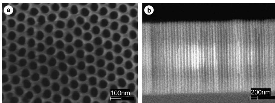
Fig. 2. The SEM picture of the nanoporous alumina sample A30 from a surface (a) and a side view (b). The size of pores and a period of the array were similar for all the investigated samples. Since it was hard to mount the sample perfectly aligned to the electron beam during the characterization, one of the side surfaces can be seen in the image (gray color).
