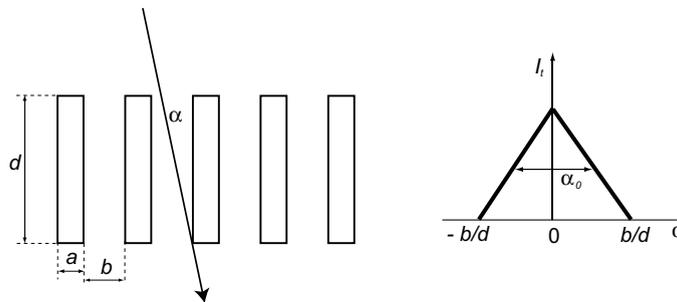
Fig. 8. A simplified model of nanoporous alumina and the expected angular dependence of transmitted current on the energy of the incident beam. The acceptance angle  $\alpha_0$  is defined as FWHM of the peak.
