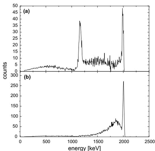
Fig. 5. Transmission energy spectrum of the samples A39a (a) and A39b (b) taken from the same alumina membrane. Bottoms of the pores at the piece A39a were not completely open, therefore the sample A39b was exposed to additional etching in  $\text{H}_3\text{PO}_4$  solution. It can be seen that the low energy peak corresponding to transmission through the solid material is broader and shifted to higher energy  $\sim 1860$  keV (b).
