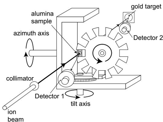
Fig. 1. Experimental setup used for the analysis. Detector 1 – the standard RBS detector, Detector 2 – the RBS detector for transmitted ions.
