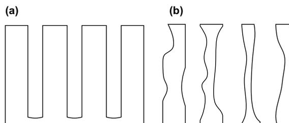
Fig. 10. Simplified sketch showing the influence of etching in the  $\text{H}_3\text{PO}_4$  solution on the sample structure. The procedure opens the pore ends after the anodization steps, but also removes solid material along the wall.
