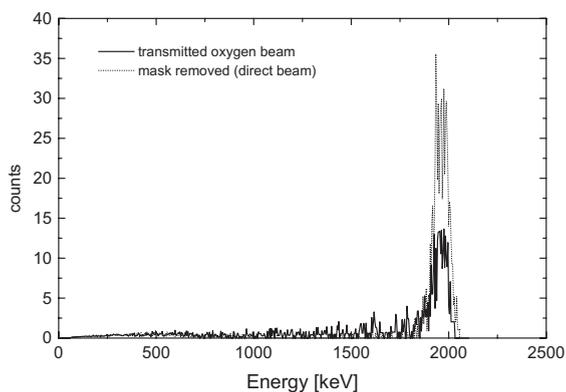
Fig. 6. Comparison between the energy spectrum of the transmitted  $\text{O}^+$  beam through the sample A30\* and the energy distribution measured with a sample removed. The resolution of these spectra is limited by the thickness of Au foil used in the detection system (Fig. 1).
