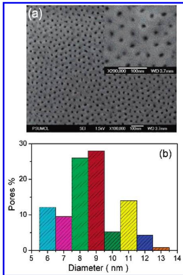
**Figure 5.** (a) FESEM image of AAO grown on an Al foil with 3 vol % H<sub>2</sub>SO<sub>4</sub>, anodized at 16 V and 0–3 °C after selective etching and detachment. The surface of the AAO was milled by an Ar ion beam for 10 min. (b) Plot of distribution of pore diameters determined from Figure 5a; 76% of the pores are below 10 nm in diameter.
