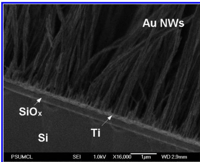
**Figure 4.** FESEM image of high-density Au nanowire array or bundles grown with an AAO film on a Ti/SiO<sub>x</sub>/Si substrate, where the AAO film was completely dissolved with 5 M NaOH solution.
