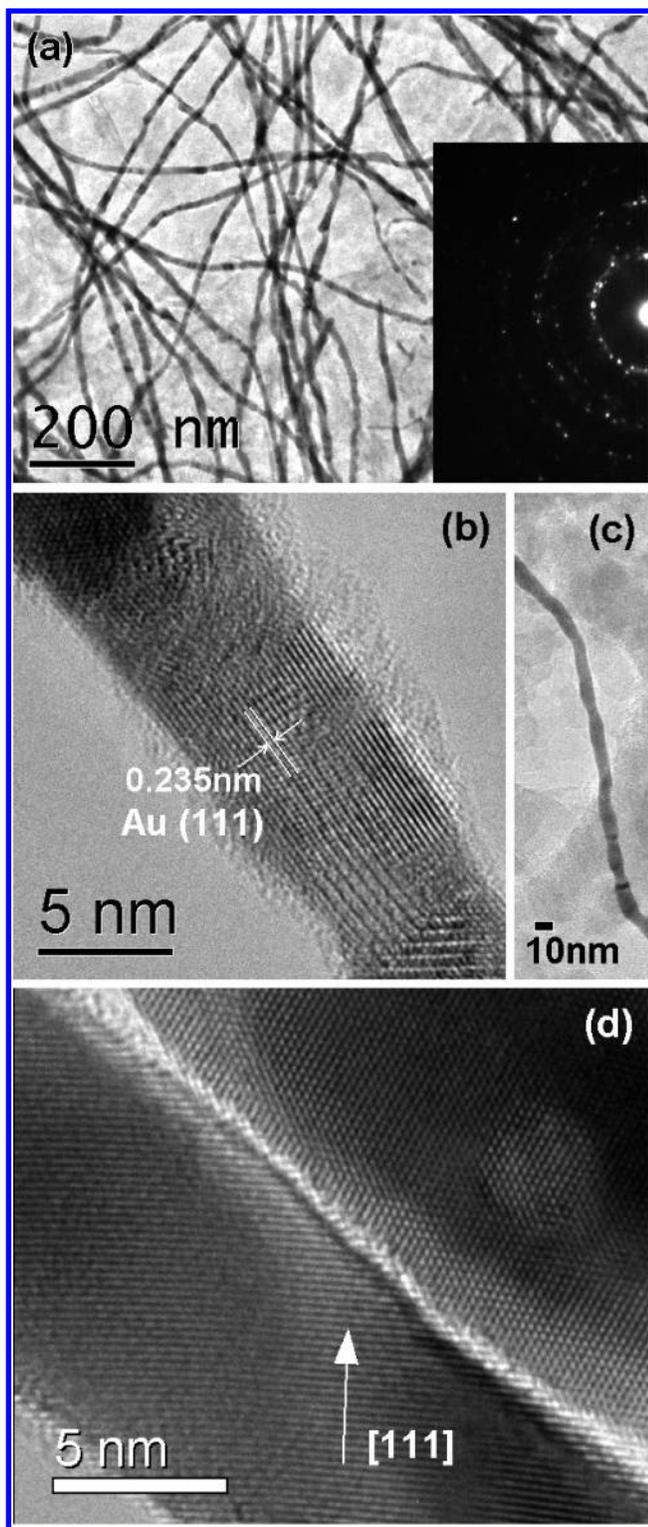
**Figure 7.** (a) Low-magnification TEM image of Au nanowire bundles and a SAED pattern. b and c, respectively, show HRTEM and low-magnification TEM images of a thin 7.2 nm Au wire. (d) HRTEM image of two selected Au wires of diameters 9–11 nm. All of the wires were made from the small-pore free-standing AAO membrane shown in Figure 5.
