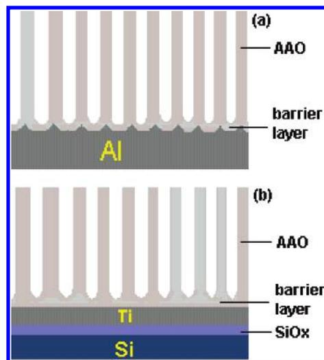
**Figure 1.** Schematic of the cross section of porous anodic alumina (AAO) films grown on (a) an aluminum foil substrate and (b) a Ti/Si<sub>x</sub>O/Si wafer.
