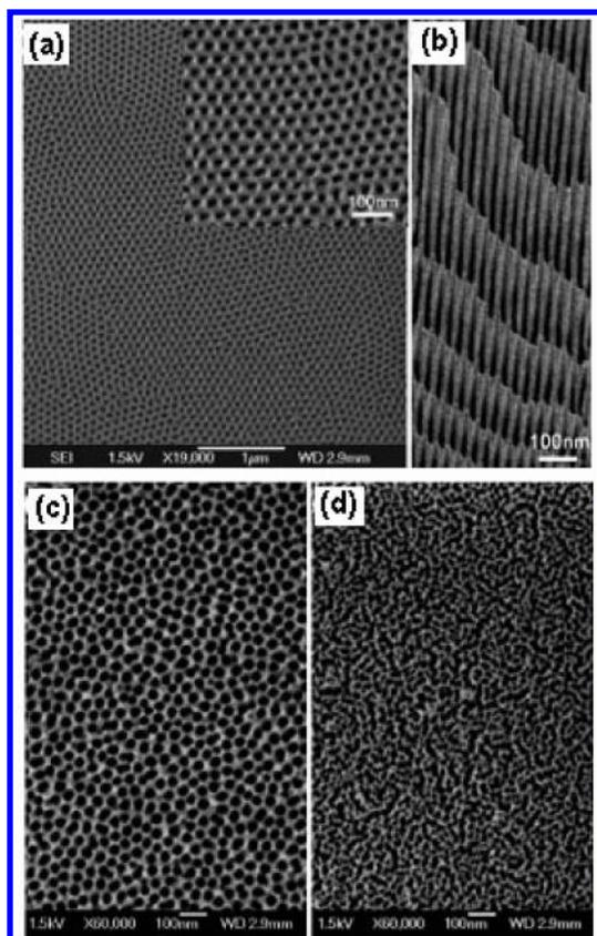
**Figure 6.** FESEM images of a free-standing AAO film anodized at  $-22$  V and  $0-3$  °C from an Al foil and detached by the reversed-bias method. (a) Bottom surface after ion milling. (b) Cross-sectional image of the film. (c) Original top surface. (d) Original bottom surface.
