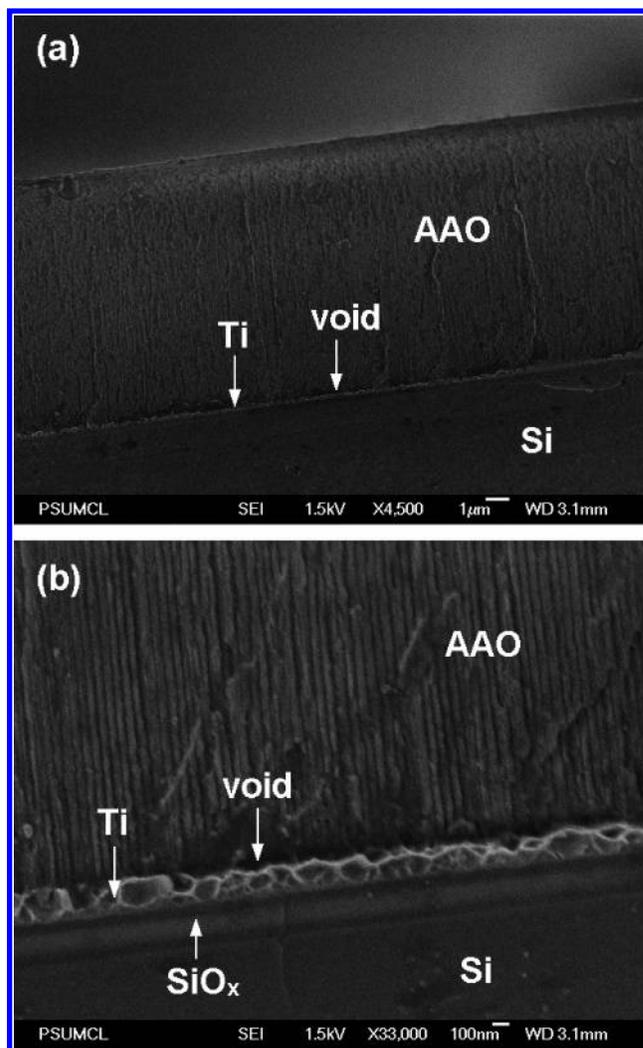
**Figure 3.** FESEM images of the cross section of the same AAO/Ti/ $\text{SiO}_x/\text{Si}$  sample shown in Figure 2, after the reversed-bias process at –3.5 V for 10 min, showing penetration of the oxide barrier layer and cracks or voids at the AAO/Ti interface: (a) low-magnification image; (b) high-magnification image.
