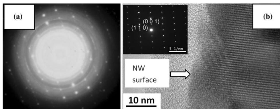
**Fig. 3** **a** SAED pattern of a Gd as-implanted nanostructure. **b** HRTEM image of a nanostructure implanted with Gd and annealed at 1100 °C. The inset shows the SAED pattern, showing a [110] zone axis
