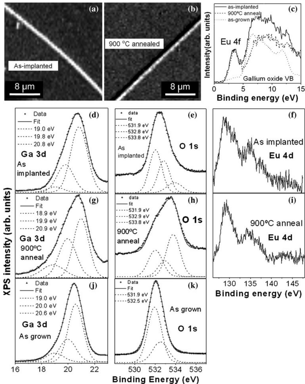
**Fig. 4** XPS results for Eu-implanted samples. **a** XPS map of the Ga 3d line from an as-implanted nanowire **b** XPS map of the Ga 3d line from an implanted and 900 °C annealed nanowire. Local XPS spectra from these nanowires are shown in figures (c)–(i) for valence band,
