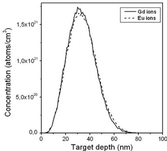
**Fig. 2** Ion concentration profile obtained with SRIM simulation for the Eu (dashed line) and Gd (solid line) implantation conditions used in this work in gallium oxide. Almost identical profiles are obtained for both ions
