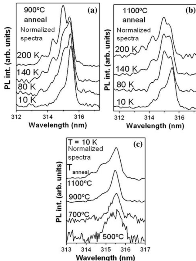
**Fig. 6** **a** PL spectra acquired at different temperatures from Gd-implanted nanowires annealed at 900 °C. **b** PL spectra acquired at different temperatures from nanowires annealed at 1100 °C. **c** PL spectra acquired at  $T = 10$  K from samples annealed at 500, 700, 900, and 1100 °C. All spectra are normalized.  $\lambda_{\text{exc}} = 248$  nm
