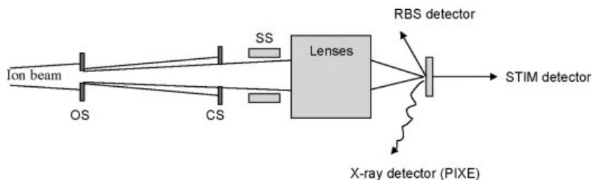
Fig. 1. Schematic of the basic components of a nuclear microprobe focusing system. OS, object slits; CS, collimation slits; SS, scanning system for beam deflection.
