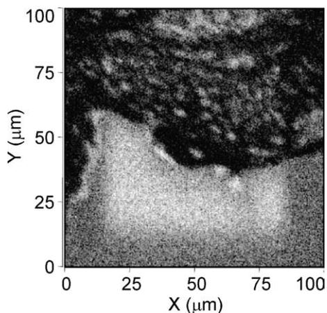
Fig. 4. On-axis STIM image of skin sample obtained during a  $150 \times 150 \mu\text{m}^2$  scan where a previous scan of  $100 \times 100 \mu\text{m}^2$  was performed. The PIPS detector damage area can be identified.
