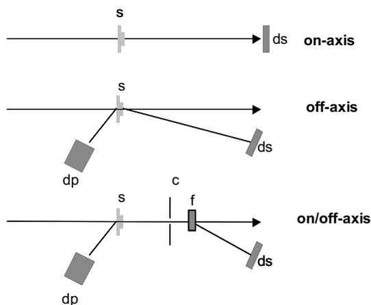
Fig. 1. Schematised STIM geometries. dp – PIXE detector, ds – STIM detector, s – sample, c – collimator, f – scattering foil.
