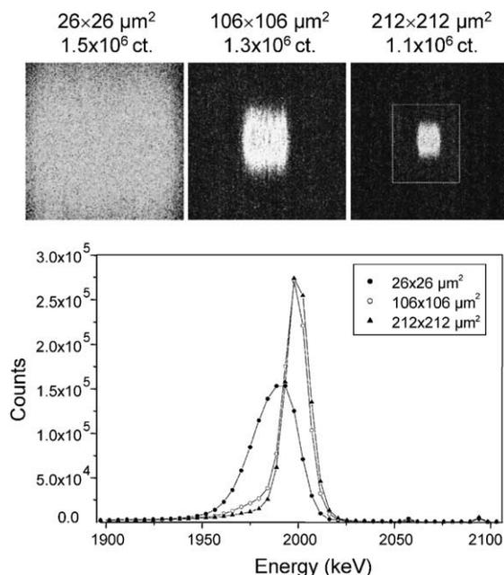
Fig. 3. Results of a direct irradiation with a 2.0 MeV proton beam of a PIN diode located at 40 mm from the focal plane after three consecutive beam scan amplitudes. The induced detector beam damage as well as the alteration in the detector response function are shown.
