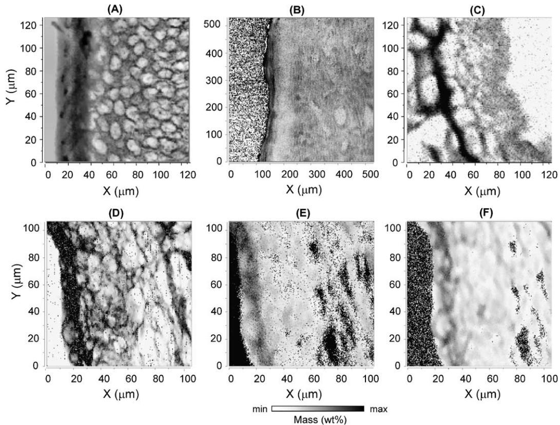
Fig. 2. Images obtained for on-axis STIM, off-axis STIM, and on/off-axis STIM geometries at different groups. (A) 14  $\mu\text{m}$  section of mouse foot sole skin, on-axis STIM at Bordeaux; (B) 25  $\mu\text{m}$  section of pig skin, off-axis STIM at Debrecen; (C) 14  $\mu\text{m}$  section of pig skin, on/off-axis STIM at Lund; 14  $\mu\text{m}$  section of pig skin, observed for the three STIM geometries (Lisbon); (D) on-axis; (E) off-axis and (F) on/off-axis.
